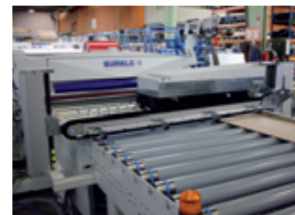
Heizzone zur Plattenvorwärmung Heating zone to pre-heat the boards
